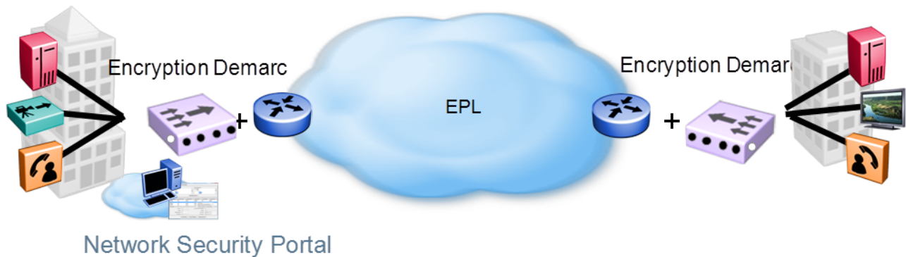
Network Security Portal, Encryption device with an Ethernet Private Line Service (EPL)
